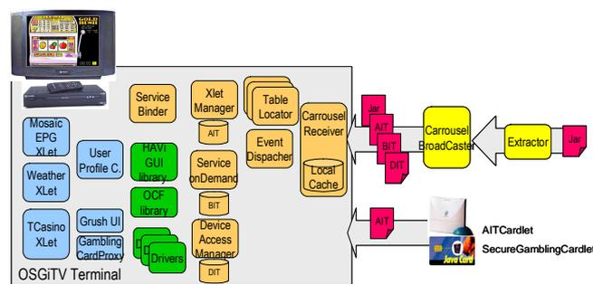
Fig 2 : Architecture of the OSGiTV deployment subplatforms.
