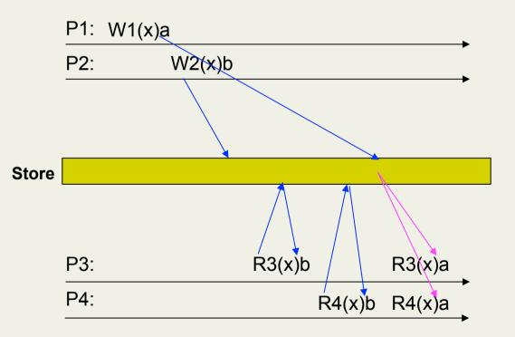
Different possible equivalent sequential orders, as if executed by a single processor, on the same memory content
