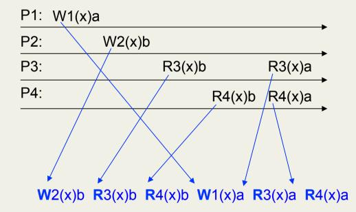
Different possible equivalent sequential orders, as if executed by a single processor, on the same memory content
