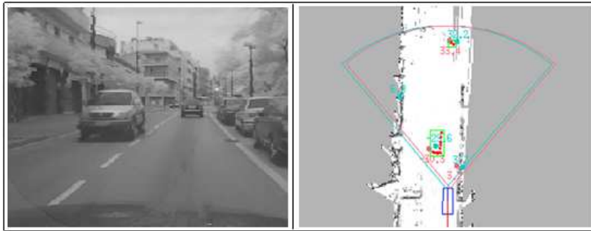
Fig. 8. Moving object detected from laser data is confirmed by radar data.
